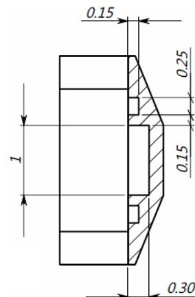
Figure 4. Dimensions of the Sliding Hall Probe (SHP). All measures are in millimetres (mm). The maximum tolerances:
