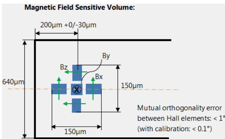
Figure 5. Overall magnetic field sensitive volume (MFSV) of the applied fully integrated 3D Hall sensor
