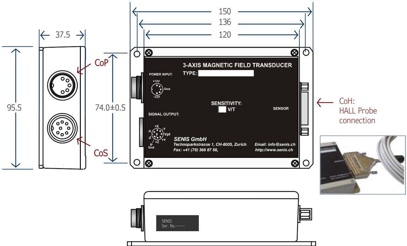
Figure 7. Dimensions and tolerances of the 3-channel analog processing module type A.1T25KJ
