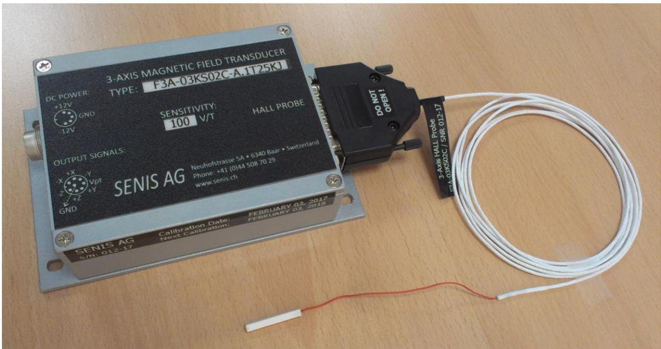
Figure 2. 3-axis magnetic field transducer type F3A-03KS02C-A.1T25KJ
