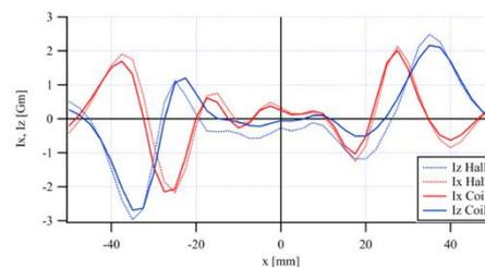
Figure : Comparison of the first field integral measurements with flip coil and Senis A.G. Ultra low Noise Transducer. This hall probe has an excellent stability due to low noise and minimal drift. It can be seen from the graph that corrections of hall probe scan with the measured flip-coil field integrals is no longer necessary. This is unique property of the Senis hall probe transducer.
