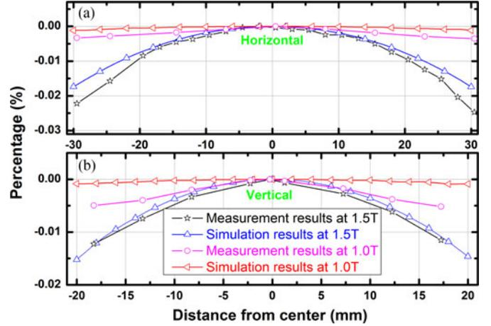
Fig. 5. Dipole magnet good field region as determined by measurements and simulation in (a) the horizontal and (b) the vertical directions.
