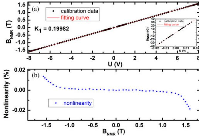
Fig. 8. (a) Field calibration data and (b) nonlinearity of the SENIS probe.
