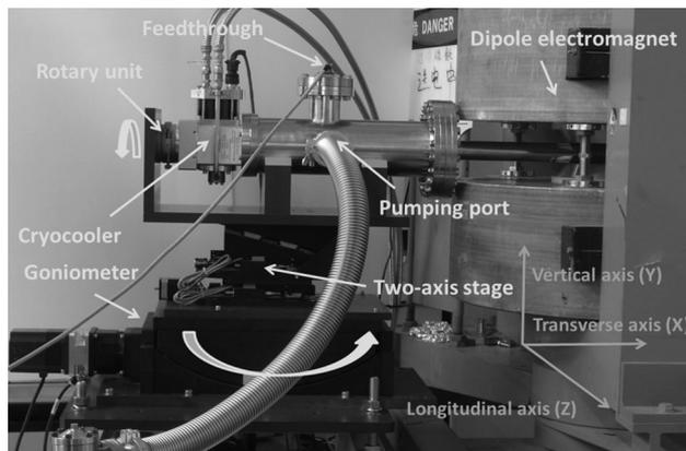
Fig. 1. Setup of the low temperature Hall probe calibration system.
