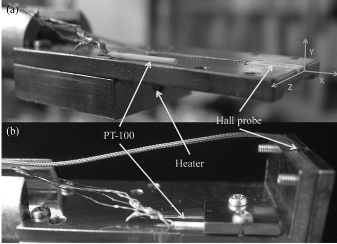
Fig. 2. Hall probe holders, heater, and PT-100 for (a) the Y channel probe, and (b) the X channel probe.
