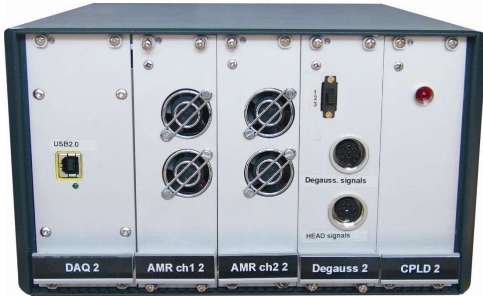
Figure 4: MiAEI02-2, dimension (W x H x D) 213,6x133.3x315.5mm
