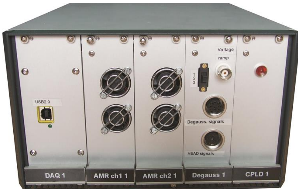
Figure 3: MiAEI02-1, dimension (W x H x D) 213,6x133.3x315.5mm
