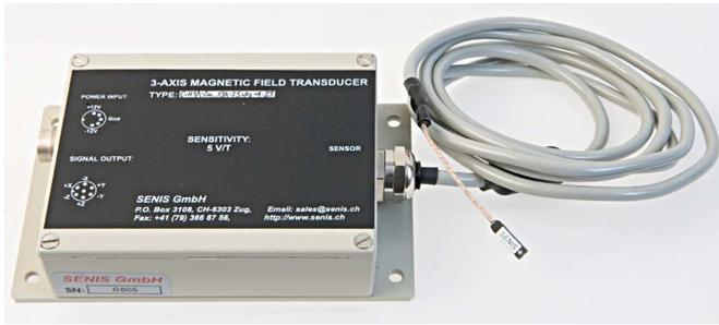
Fig. 2. SENIS analog three-axis Hall magnetic field transducer. With reference to Fig. 1, module E (the box) and module H (the cable with the Hall probe) are visible. The front end of the cable is very thin and flexible to allow easy positioning of the probe.
