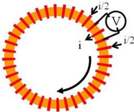
Figure 3: Principle of the circular vertical Hall device (CVHD). The ring represents a narrow n-well region, and the radial bars are the N<sup>+</sup> contacts. An array of integrated CMOS switches (not shown) connects sequentially a set of 5 contacts, so that the 5-contact vertical Hall device virtually moves along the ring.
