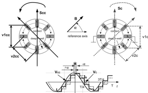
Figure 4: Biasing and sensing of the Hall voltages of the two 8CVHDs. Low-middle figure: clockwise (dashed line), counter clockwise (full line) and the band-pass filtered signals for the DC magnetic field enclosing the angle  $\alpha$  with the reference axis.
